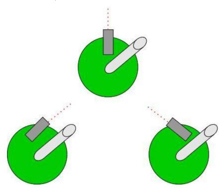
The diagram above shows the organization of our Roomba flock-swarm. The dark grey boxes represent our omni-directional LIDAR. To allow the LIDAR to locate other bots we will use long pvc pipes, represented as light grey cylinders above, as reliable markers for the sensors to identify. Since they will be the same size we can configure the robot to reliably identify that marker and track it for relative position.
